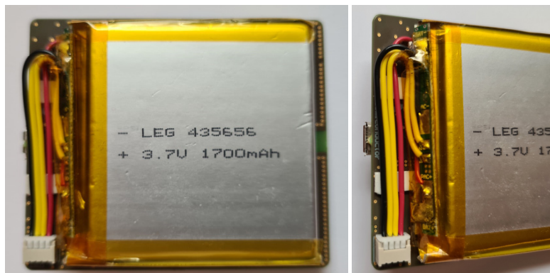
Figure 12. Physical Implementation of the Battery and its Protection Circuit from Bottom Side of SECO-RSL10-CAM-GEVB
