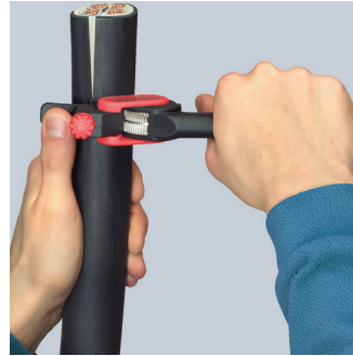
Turning the tool for circumferential cut
