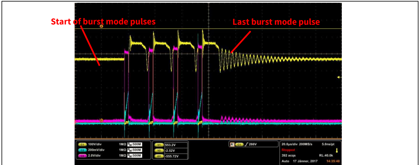
Figure 20 High line (265 V AC ), no load. The ICE2QS03G is operating in burst mode to minimize idle power consumption. The burst mode pulse train shown above occurs every 33.8 ms. QR valley switching does not occur during burst mode due to the ICE2QS03G changing operating modes at light load. V DS maximum is only 553 V in burst mode operation.
