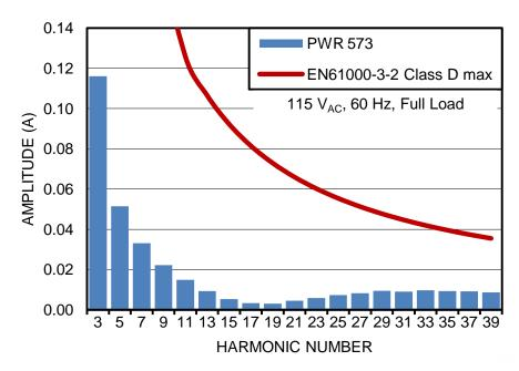
Figure 10. UCC28180EVM-573 Current Harmonics, (115-V<sub>AC</sub>, 60-Hz input, full load, without the fundamental)
