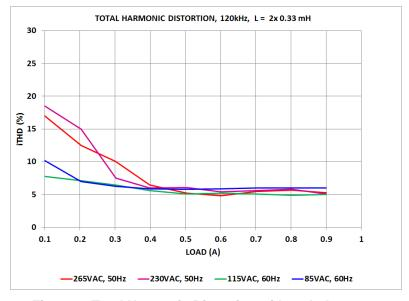
Figure 6. Total Harmonic Distortion with 2x Inductance
