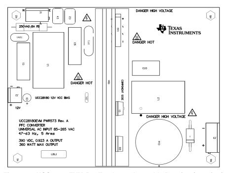
Figure 22. UCC28180EVM-573 Top Layer Assembly Drawing (top view)
