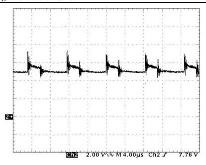
Figure 15. UCC28180EVM-573 Switching Frequency Output Voltage Ripple (115  $V_{AC}$ , 60 Hz input, full load)
