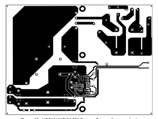
Figure 25. UCC28180EVM-573 Bottom Copper (bottom view)
