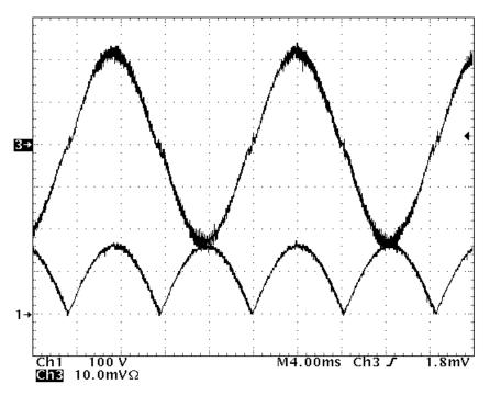
Figure 11. UCC28180EVM-573 Input Current and Input Voltage at the Output of the Bridge Ruectifier, (115- $V_{AC}$ , 60 Hz, full load. (CH 1 = rectified input voltage on BR1, 100 V/div., CH 3 =  $I_{IN}$  2 A/div.))
