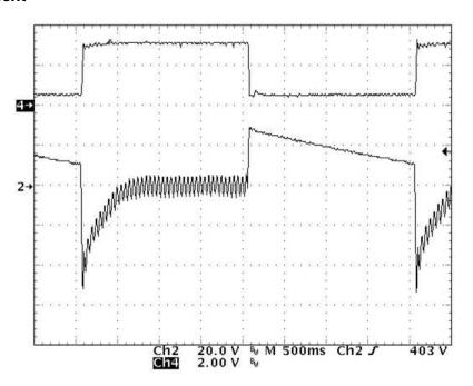
Figure 19. Load Transient (115 - $V_{AC}$ , 60-Hz, load step: 0% to 100%. Ch 2 =  $V_{OUT}$  at 20 V/div., offset by 386 V, Ch.4 =  $V_{COMP}$  at 2 V/div)
