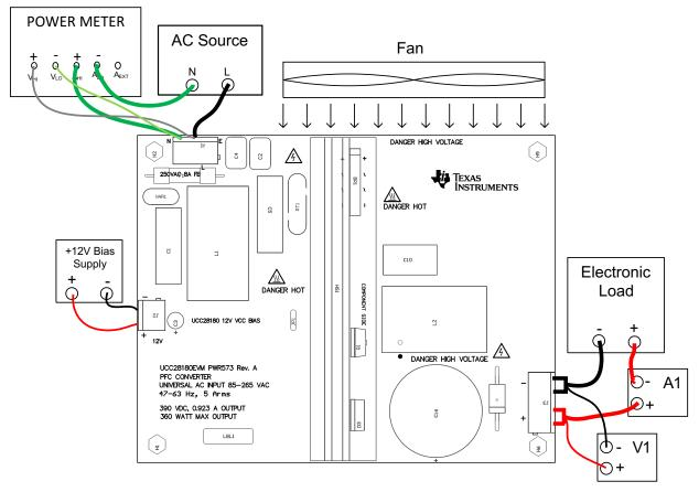
Figure 2. UCC28180EVM-573 Recommended Test Set Up
