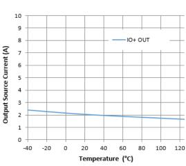
Figure 13. Output Source Current vs. Temperature
