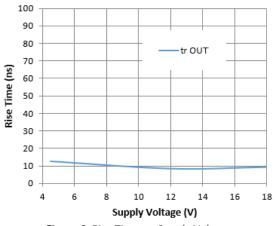
Figure 6. Rise Time vs. Supply Voltage
