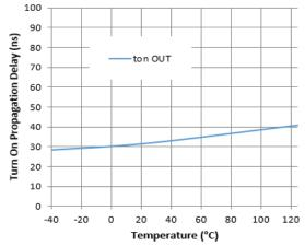
Figure 3. Turn-on Propagation Delay vs. Temperature
