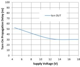
Figure 2. Turn-on Propagation Delay vs. Supply Voltage
