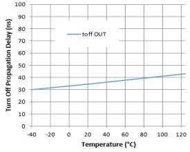
Figure 5. Turn-off Propagation Delay vs. Temperature
