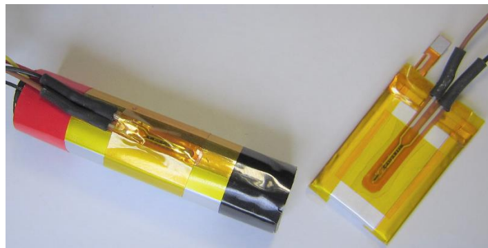
Figure 7. A LEAD TYPE THERMISTOR MOUNTING
