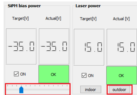
Figure 14. SiPM Bias Voltage Reduction (Clicking Outdoor Button or Using the Slider ) Helps to Achieve OK Status at High Ambient Illumination
