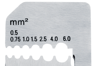
12 21 180: wire cross-sections in mm 2
