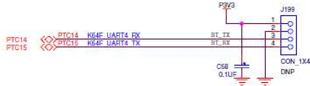
Figure 17. Add-on Bluetooth module
