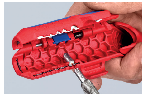
Stripping the internal portion of the coax cable
