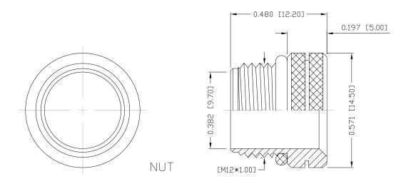
NOTE: MATERIAL HOUSING: PBT UL94V-0, BLACK BRASS CONTACT: NUT: BRASS D-RING: EPDM, BLACK FINISH CONTACT: GOLD PLATED OVER 504" NICKEL NICKEL PLATED NUT: 60ц" ТО 100ц" OVER ALL ELECTRICAL RATED CURRENT: 4Α 250V RATED VOLTAGE: 100 MOhms MIN.
