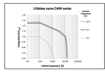
V = Operating Voltage [VAC] V<sub>rms</sub> = Rated Voltage [VAC]
