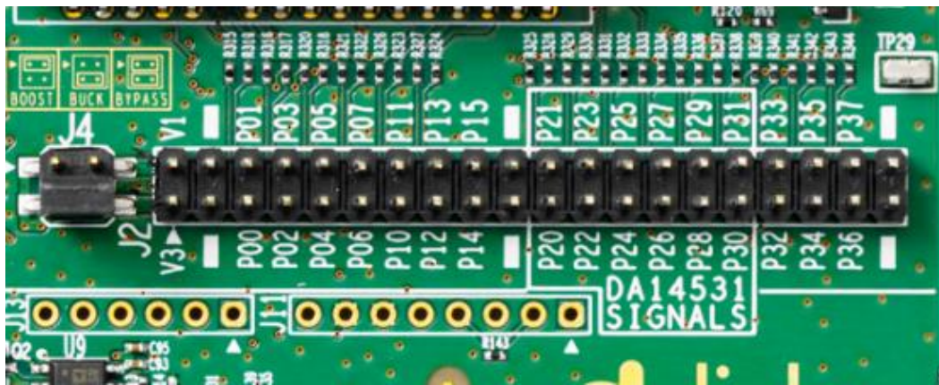
Figure 18: J2, Breakout Header of DA14531 PRO-MB
